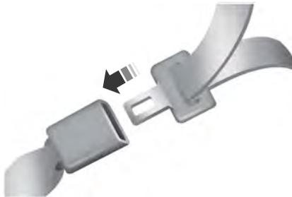
1. Insert the belt tongue into the proper buckle (the buckle closest to the direction the tongue is coming from) until you hear a snap and feel it latch. Make sure you securely fasten the tongue in the buckle.
