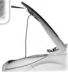
4. Open the hood. Support the hood with the strut.
